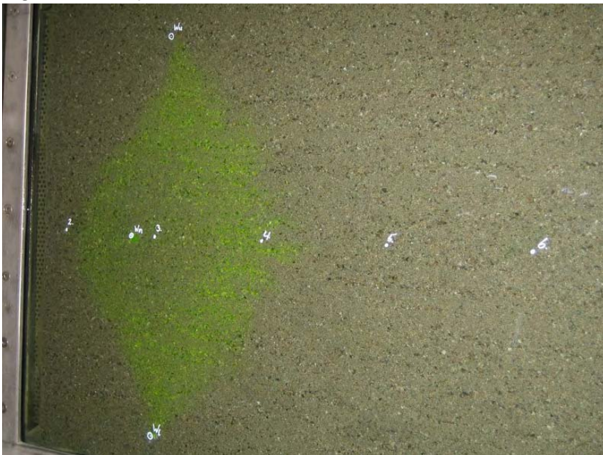
Fig. 2.3: Injection, extraction with dye tracer test
