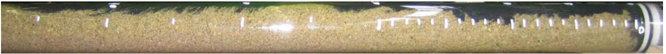
Fig. 3.20: Preferential flow path resulting from a bend through of the column before injection
