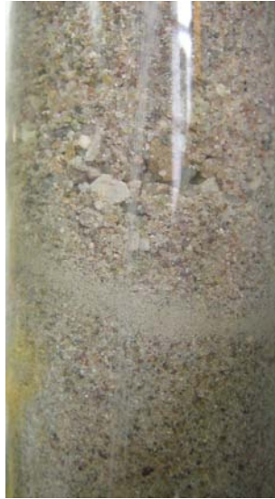
Fig. 3.19: Small heterogeneities that can occur during packing with material of a large grain-size distribution, here a small coarse and fine grained layer are visible
